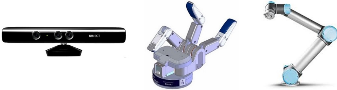
Figure 5.11: Robot hardware components: (left)Microsoft Kinect, (middle) Barrett Hand, (right) UR5 arm
