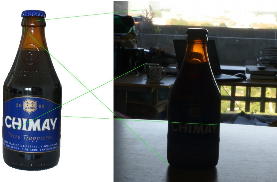
Figure 2.1: Model matching failure in underexposed 2D images. None of the features extracted from the model (left) can be successfully matched onto the object of interest (right)(image from https://pointclouds.org/ ).
