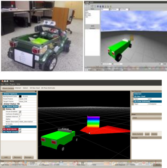
Fig 5. The model of our mobile robot ANT. From left to right and top to bottom: Robot model in real time, Robot model in Gazebo, Robot model and point cloud visualization in Rviz
