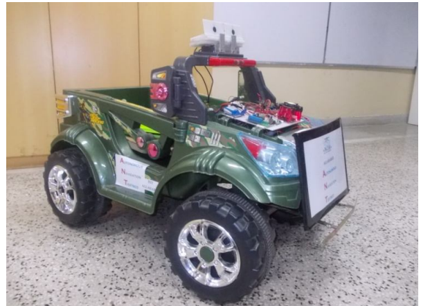
Fig. 1. The ANT (Autonomous Navigation Testbed) mobile robot used for the purpose of experiments of this paper.
